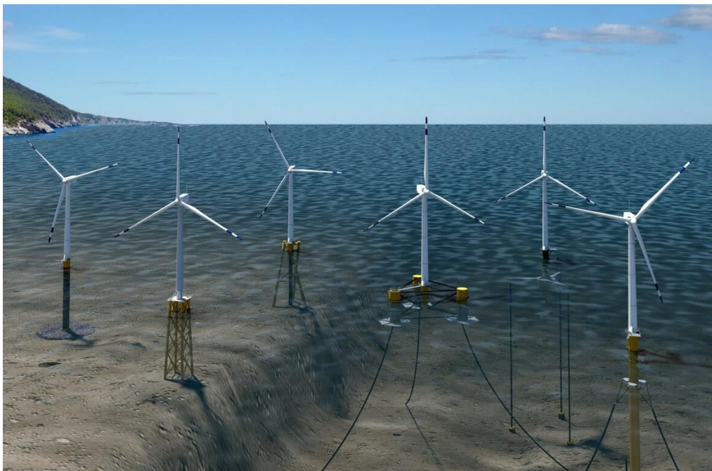
Offshore wind foundation types. From left to right: monopile, jacket, twisted jacket, tension-leg floating platform, semi-submersible platform, and spar-buoy. Credit: National Renewable Energy Laboratory .
